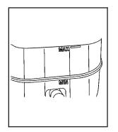
Look at the brake fluid reservoir. The fluid level should be above MIN. If it is not, have your brake system checked to see if there is a leak.
